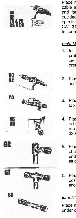
Place mold against surface with end of cable under center of tap hole#1 AWG and larger cables require the use of packing material to seal the mold cable opening. Use the handle or Cat. No CAT-340 Chain Clamp to secure mold to surface.
